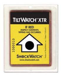
The TiltWatch XTR is single-use tip indicator used to monitor goods that must remain upright to insure intact delivery. The device continual monitors shipments and does not activate until it is at an 80° angle +/-5% from vertical along a single plane.
